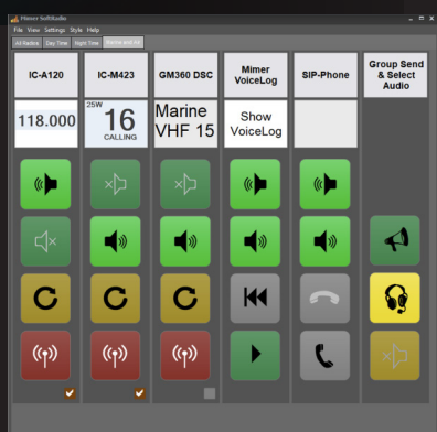
SoftRadio operator GUI with airband and marine radios as well as voice recording and phone connection.
