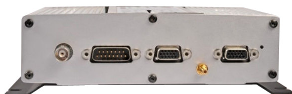
Tetra-Antenne Power/audio Interface 1 GPS-Antenne Interface 2
