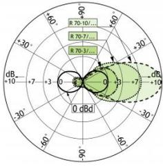
If the antennas are mounted for vertical polarization, these curves show the radiation patterns in the vertical plane.
