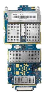
The SRB is a high performance, voice- and data-capable TETRA radio board. It provides a highly flexible and customisable TETRA engine ready to meet the requirements of third-party solution providers.
